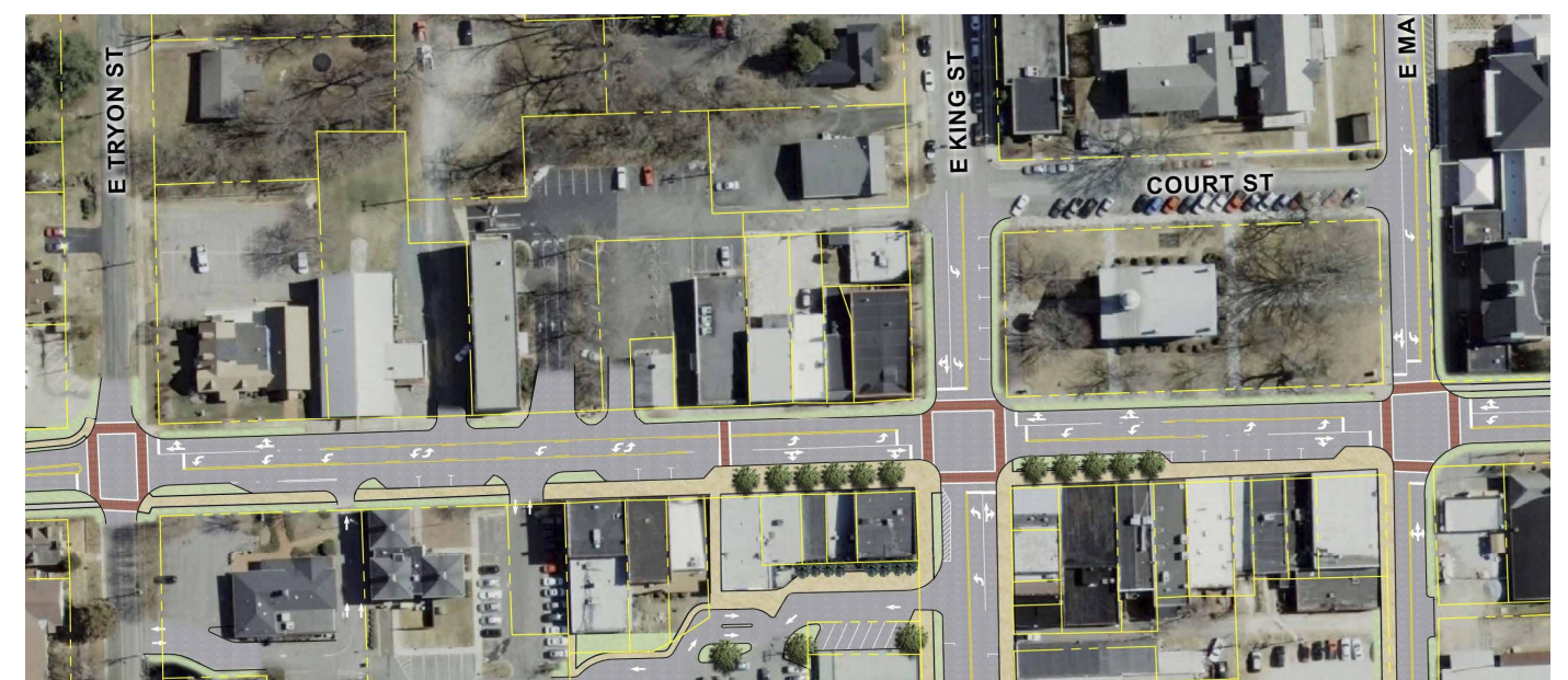
These images show laneage on Churton Street between Nash and Kollock Street and Margaret Lane (above) and Margaret Lane to Tryon Street (below). The improvements shown below will require the removal of underutilized northbound on-street parking at SunTrust.
