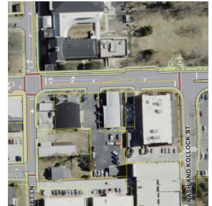
These images show laneage on Churton Street between Nash and Kollock Street and Margaret Lane (above) and Margaret Lane to Tryon Street (below). The improvements shown below will require the removal of underutilized northbound on-street parking at SunTrust.
