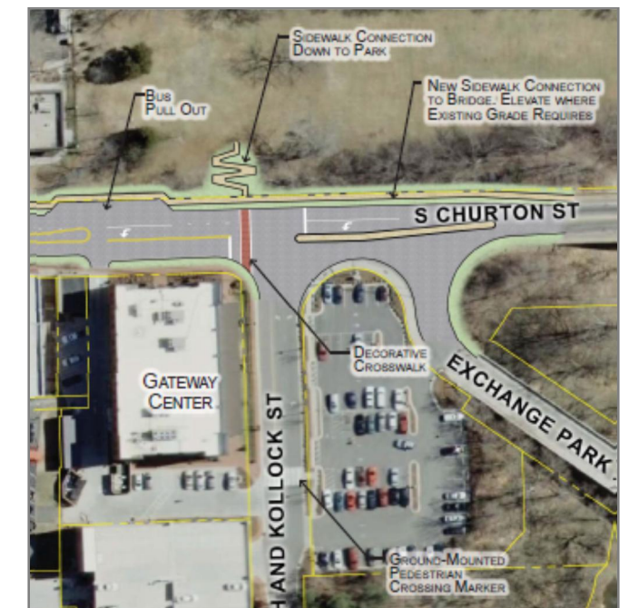
This portion of the Concept Design shows many features that aim to improve the safety and mobility for non-vehicular traffic. Improvements shown here include a sidewalk connection that fills the gap between the existing sidewalk near the Courthouse to the Eno River bridge. A decorative crosswalk at the Nash and Kollock Street signal and connection to River Park also is shown. Mid-block crossings on side streets are shown on the Concept Designs with an emphasis on ground-mounted pedestrian crossing markers.
