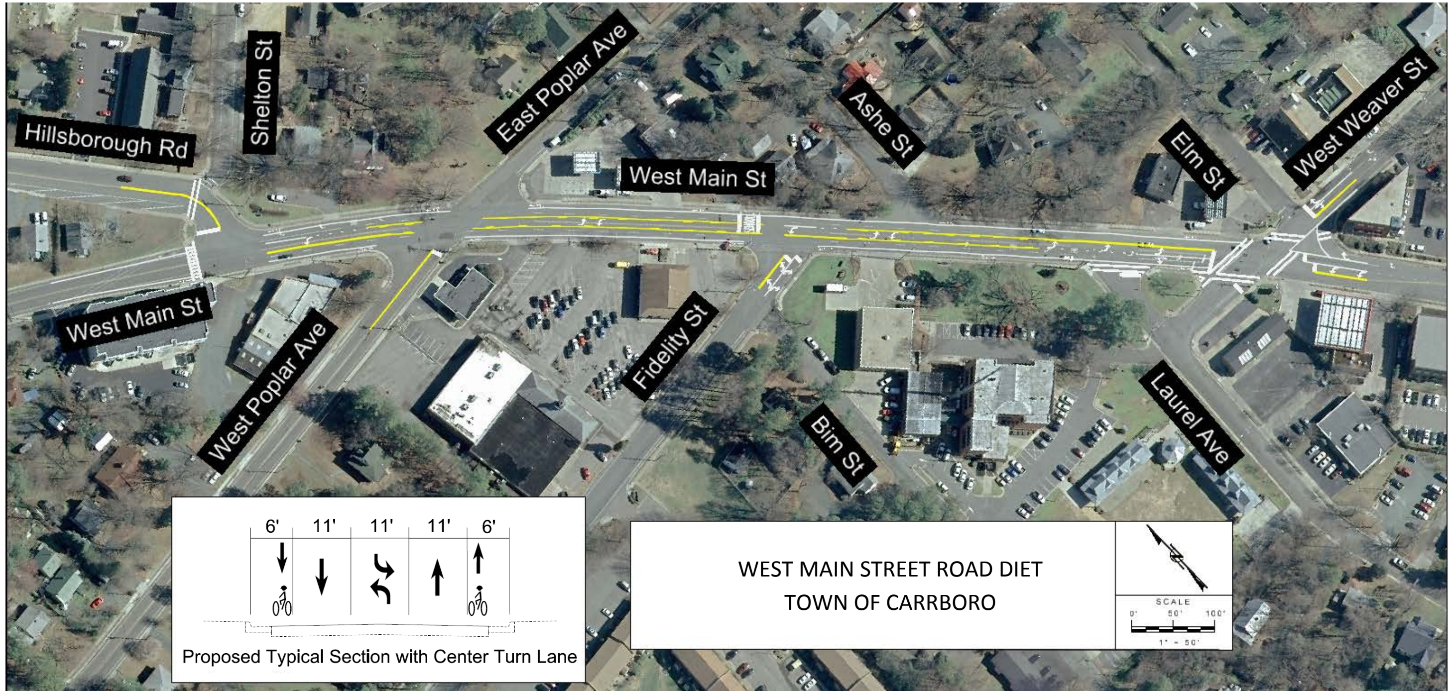
Figure 27: Road Diet Pavement Marking Plan
